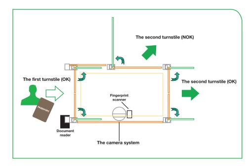
It then carries out facial recognition and/or fingerprint matching to verify the traveler's identity against the document biometric data itself, or against a biometric traveler registration database.
